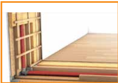
Oval pipes going through the floor, round pipes up the wall
